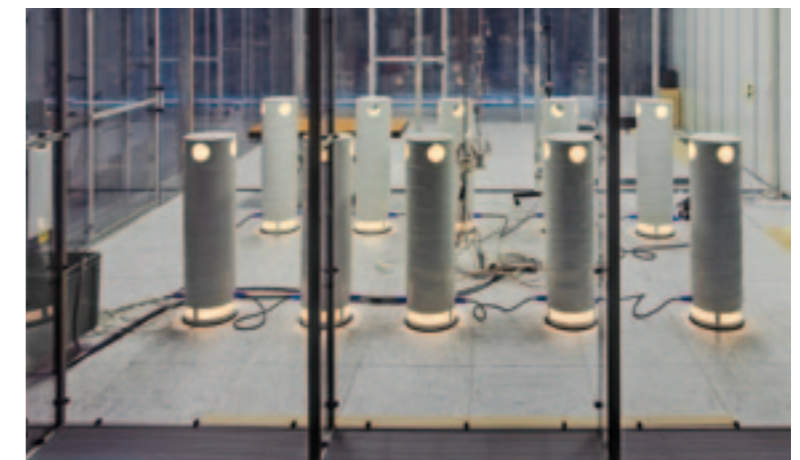
Heat and cooling output test cabin
