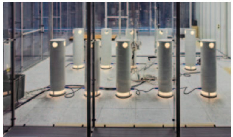
Heat and cooling output test cabin
