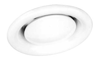
Valve adjustment is achieved by simply rotating the central core inwards or outwards on its spindle and locking into its set position using the holding nut at the rear of the valve assembly. The GXF Fire Rated Valve functions as a normal extract valve, sharing the same basic construction and performance as the GXD, however this unit also incorporates a spring
