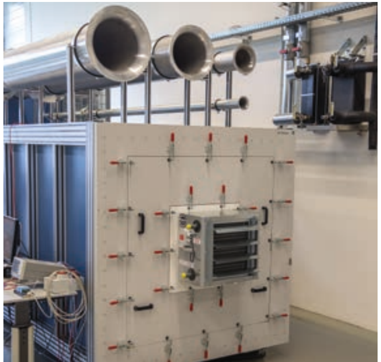
Test chamber for air performance measurements according to EN ISO 3745 (formerly DIN 24163); Kampmann R & D Centre (FEC)
